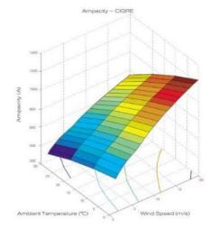
Ampacity Vs Wind Speed and Temperature
